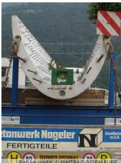
Figure 23: partly prefabricated concrete pile with non-load bearing half shells [VINTRAG INGENIEURE]
