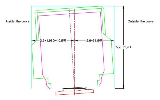
2. MIXED TRAFFIC SECTIONS STRUCTURE GAUGE (D IS THE CANT, R IS CURVE RADIUS)
