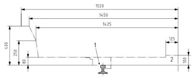
1. EXTRACT FROM EN15273-3 FOR GI3 KINEMATIC GAUGE
