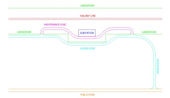
FIGURE 3 RECOMMENDED PRINCIPAL ROAD SCHEME FOR SUB-STATION
