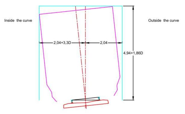
3. Passengers only and light freight traffic sections Structure gauge (d is the cant, R is curve radius)
