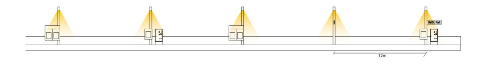
Elevation lighting principle for the platform
