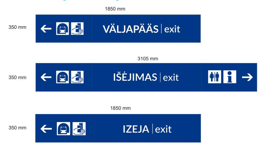
Typical dimensions of a single-line sign
