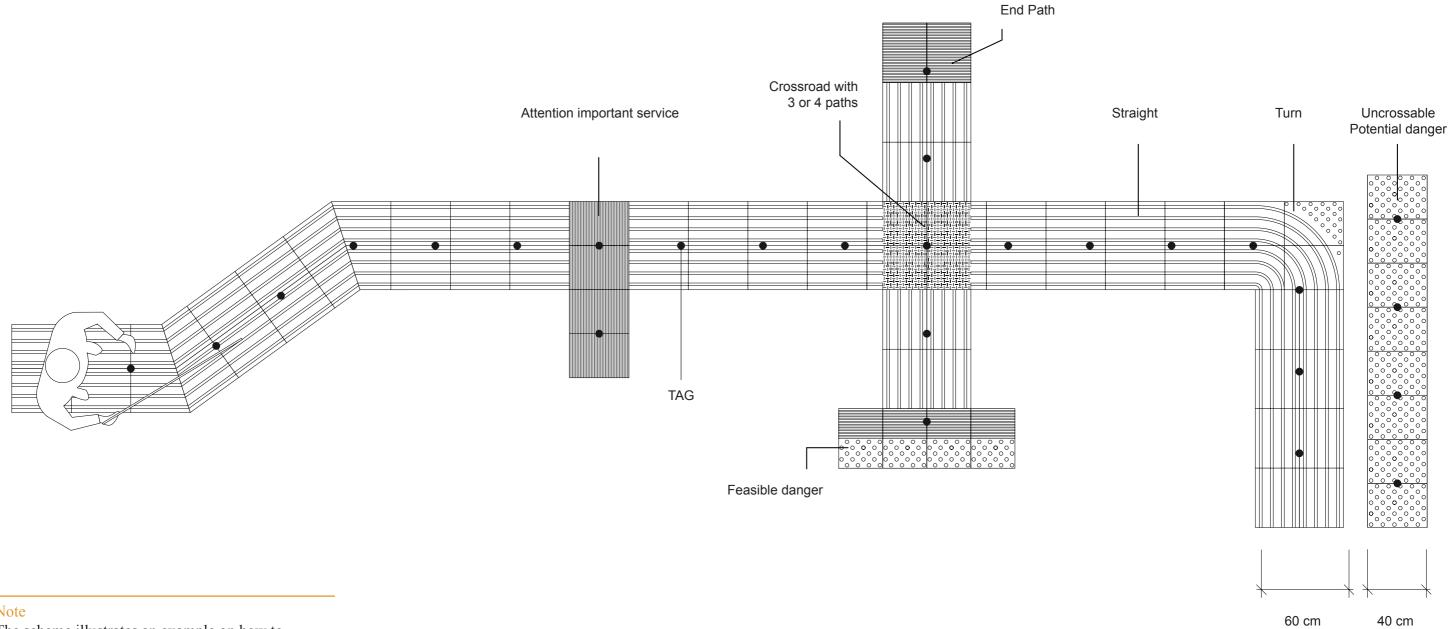
The scheme illustrates an example on how to combine the different tactile tiles.
