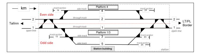
Tracks in station shall be numbered with up to three-digit Arabic numerals, however zero in the beginning of the number shall not be spelled. Station through tracks (from/to open line) shall keep its "open line" numbers, i.e. 1 or 2. Side tracks on the odd side of the station (side of the track 1) shall receive odd numbers, i.e. 3, 5, 7, etc. Side tracks on the even side of the station (side of the track 2) shall receive even numbers, i.e. 2, 4, 6, etc.
