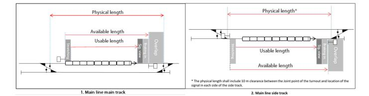
The available track length is defined considering the signalling system planned to be installed. For main tracks, the available track length is defined as a distance between the ETCS marker board or start signal for the specific direction and the ETCS marker board or start signal for the opposite direction.
