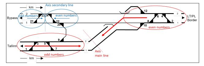
The number of the turnout, on the drawing which covers more than one station, shall be spelled with the abbreviation of the station, passing loop or crossover (talking code) which the turnout belongs to.
