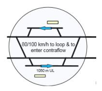
It shall be noted that this schematic allows to retain 1050m long freight trains on both the platform loops and on the passing through tracks for being overtaken by an international passenger train serving or even not serving the station. Station are fully designed on a symmetrical basis to provide the same easiness of operation when trains are running on the reverse side.
