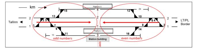
Turnouts of the crossover in station shall be numbered with two consequent numbers, e.g. 10 and 12 or 13 and 15. When spelling a crossover number, a slash symbol shall be used: 10/12 or 13/15.
