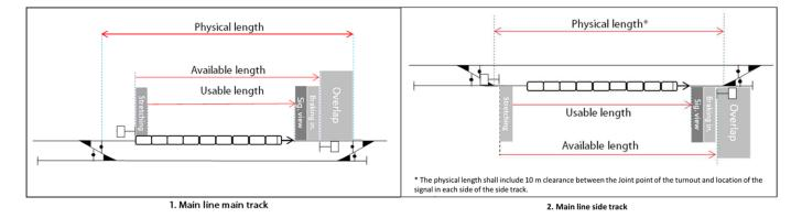
The available track length is defined considering the signalling system planned to be installed. For main tracks, the available track length is defined as a distance between the ETCS marker board or start signal for the specific direction and the ETCS marker board or start signal for the opposite direction.
