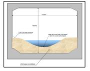
A "natural" waterbed shall be defined in the structures for vulnerable rivers with rare fish species or forming an aquatic corridor. As for the diversions, the environmental design is related to the hydraulic constrains. A 40-cm layer of material on the inside floor of the structure may be planned (see on the left the typical section of a waterbed renaturation in a hydraulic structure). The material granulometry is defined according to the stream conditions.
