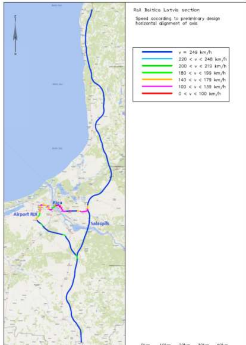
FIGURE 1: Proposed Rail Baltica alignment and maximum speeds in Latvia as per preliminary design
