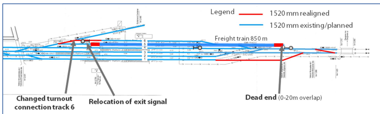
FIGURE 84: TORŅAKALNS STATION - LAYOUT PRINCIPLE WITH 850 M FREIGHT SIDING
