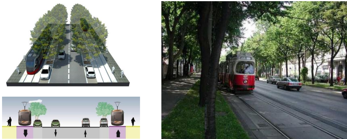
Figure 3.30: example of bilateral track position
