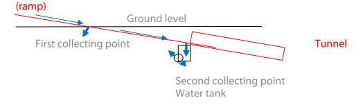
Figure 4. Ramp to tunnel drainage principle
