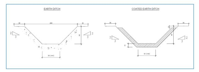
Figure 3. Typical cross section of earth ditch and coated (contrete lined) earth ditch
