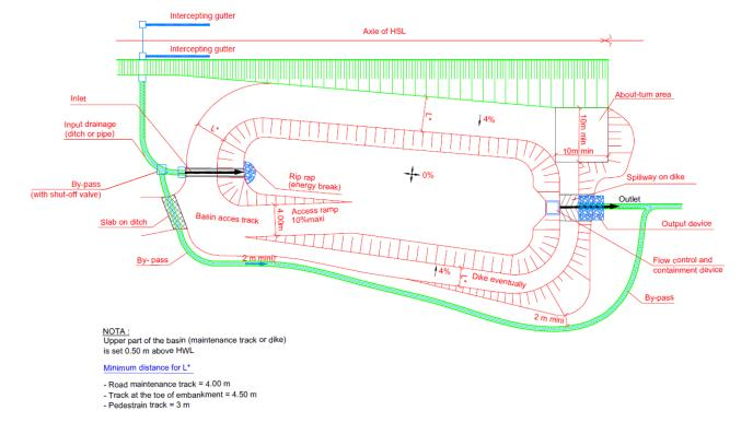
Figure 9. Containment and retention basin schema
