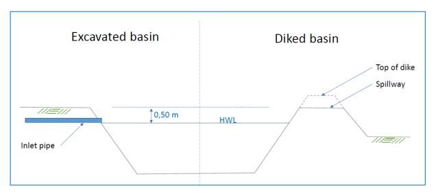
Figure 8. Relation of HWL in basin with inlet pipe and spillway
