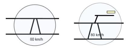
As a consequence, crossovers between the Down and Up tracks are designed every 25 km approximately to provide the ability to divert trains from one track to another at reduced speed (80 km/h on the crossover – increase to 100 km/h is possible but not mandatory). The exact requirements for speed in turnout shall be defined by the operation plan.
