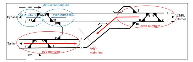
The number of the turnout, on the drawing which covers more than one station, shall be spelled with the abbreviation of the station, passing loop or crossover (talking code) which the turnout belongs to.
