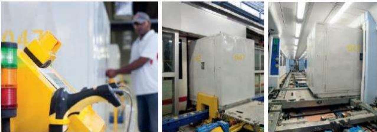
Illustration 24. Sibag solution proposed by Siemens (conveyor, container, with automatic loading into the train)
