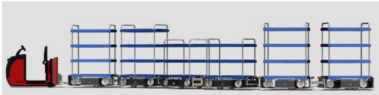
Illustration 26. Tug for the transport of containers or trolley cages with lifting system integrated in the wagon
