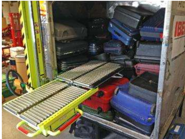
Illustration 28. Container equipped with a telescopic table
