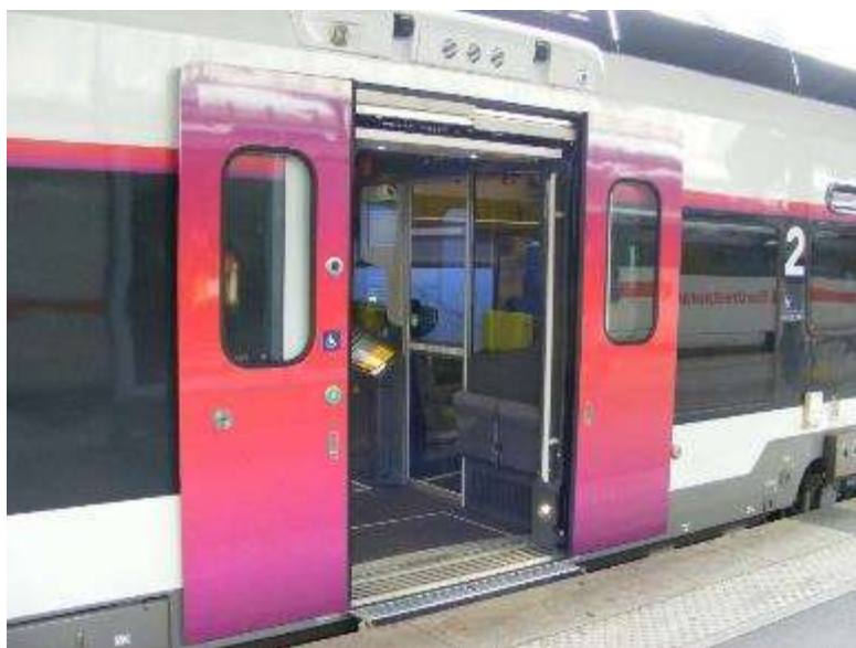
Illustration 29. Direct access to 760 mm height platform (Coradia)
