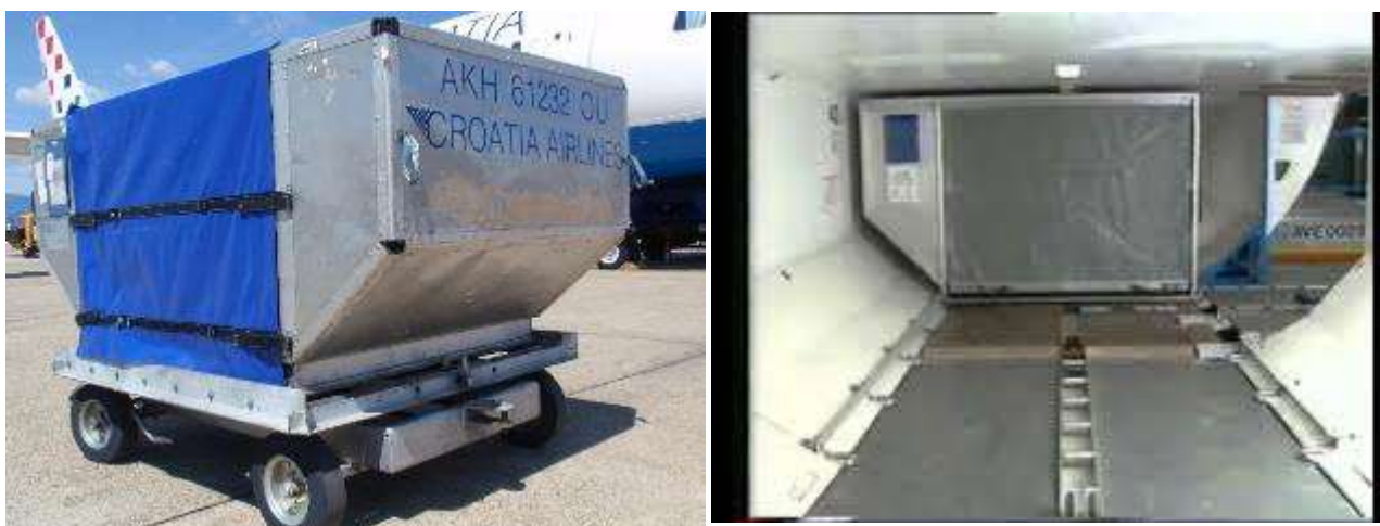
Illustration 22. Aircraft container, loaded into plane and locked
