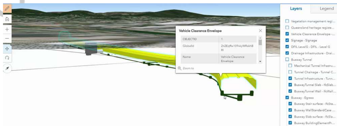
Figure 44: Example of BIM model integrated in a GIS model
